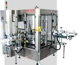
System - RS is a squared-based configuration with 3 different carousel diameters, suitable for the labelling of any type of container. It allows for the application of up to 4 labels on the same product. With its standard high-quality components, RS is ideal for lines with speeds up to 250 BPM.
