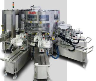
All the versatility of System-RE with a specific set-up for high-speed lines: wide carousel diameters, high-resistance size change parts, centralized automatic lubrication system. With its dedicated labelling stations Proper-3 and Proper-4, this system can handle production speeds of up to 1000 BPM with the utmost application precision.
